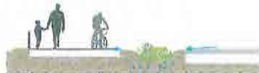
A 10' wide multi-use path with greenway features separates pedestrians and bicyclists from the road. Planted swales can help capture and slow runoff from sidewalks and roads.
